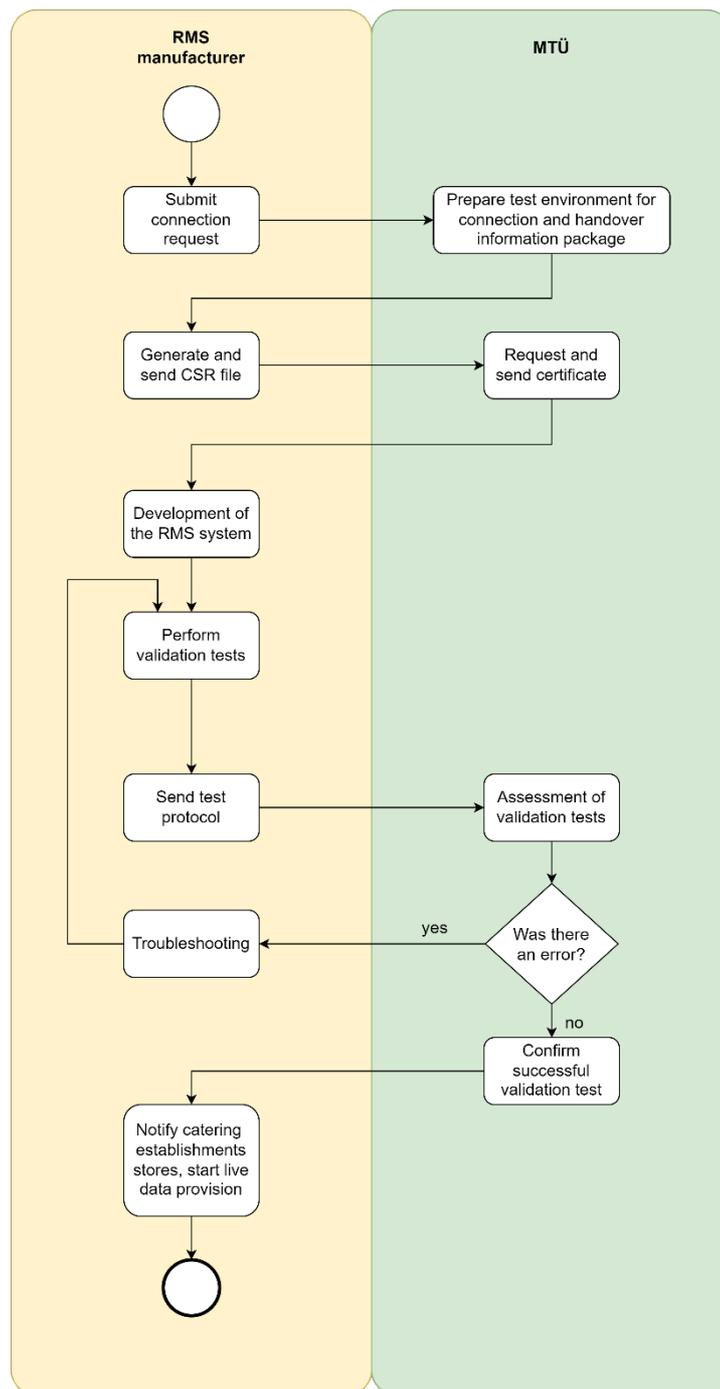
Steps of the RMS software connection process:
